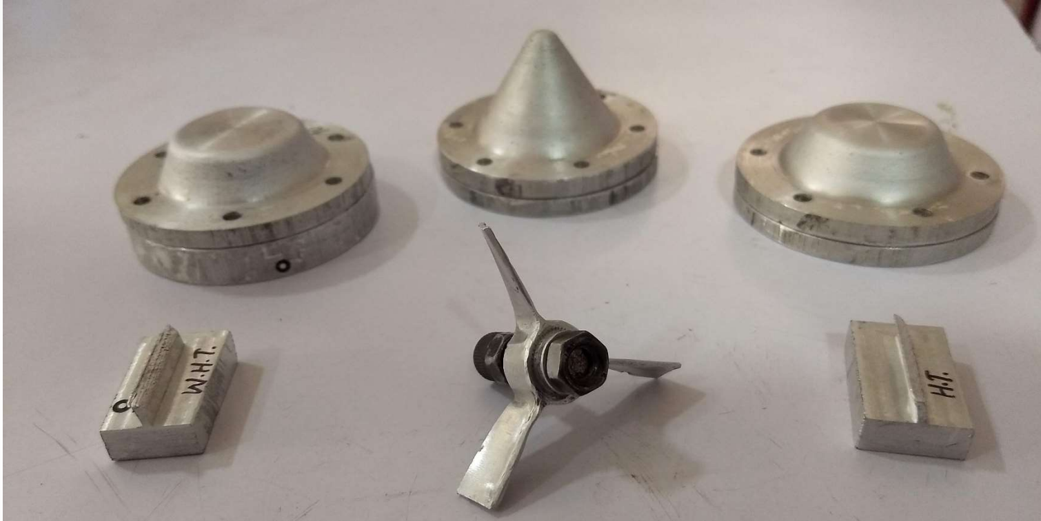
Parts Fabricated using Deformation Machining @deLOGIC Lab
