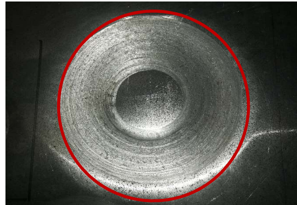
Defects in objects formed by Incremental Forming Process
