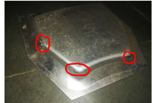
Defects in objects formed by Incremental Forming Process
