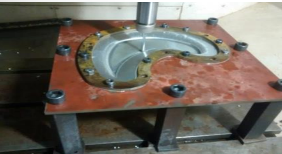
Customized clamping for custom cut blanks
