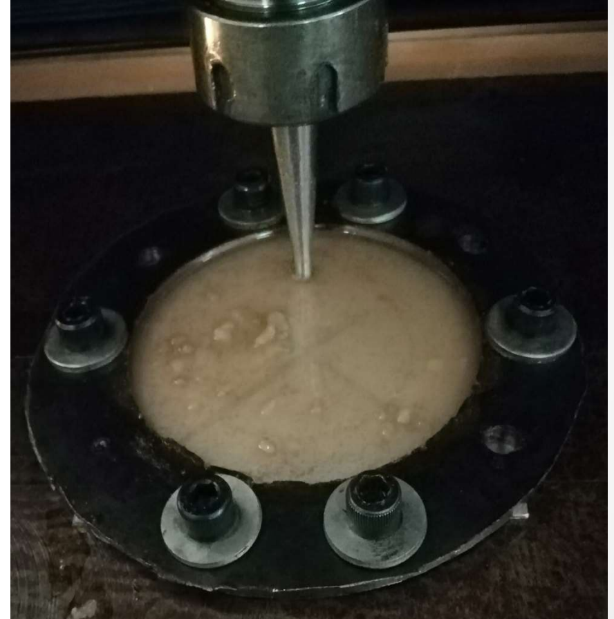
ET-IF Process with different Lubricants
