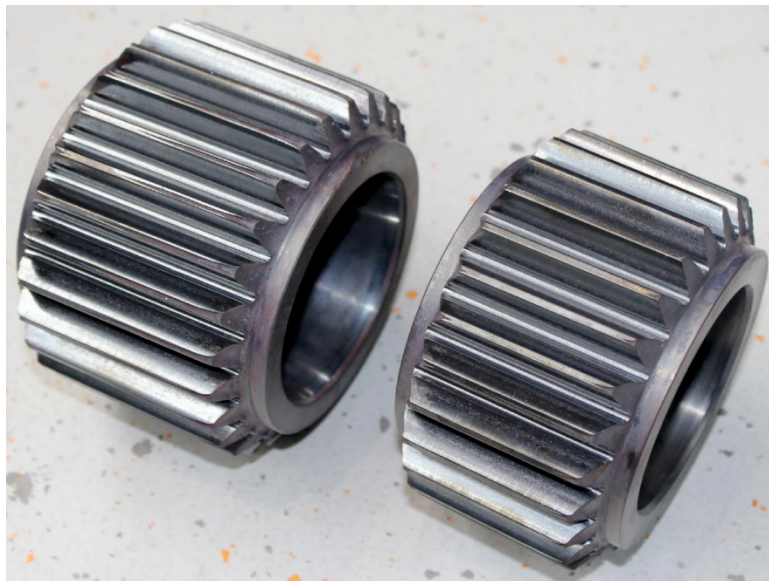
Ring Gear 18CrNiMo7-6 D_a = 122,86 \text{ mm} m = 4 \text{ mm} z = 27
