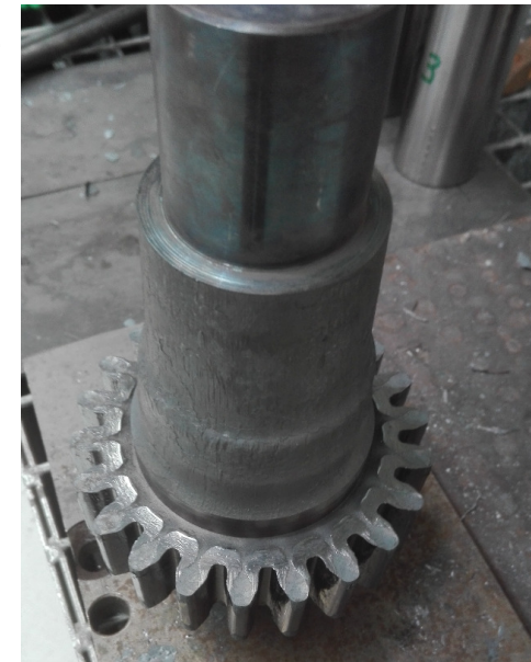
Geared Shaft 20MoCr4 D_a = 108,25 \text{ mm} m = 4,5 \text{ mm} z = 22
