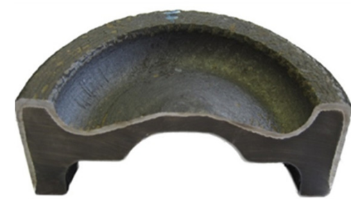
Realized piston head (D = 160 mm)
